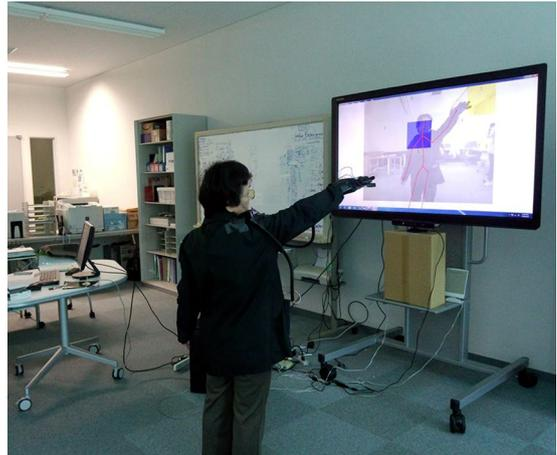
Fig.2. A visually impaired person (VIP) interacting with a large wall-mounted display using the gesture input and the haptic feedback.
