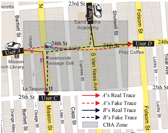
Fig.2. Example of 2-anonymity CBA zone (user A and user B each generates a fake trace to confuse each other's real paths).
