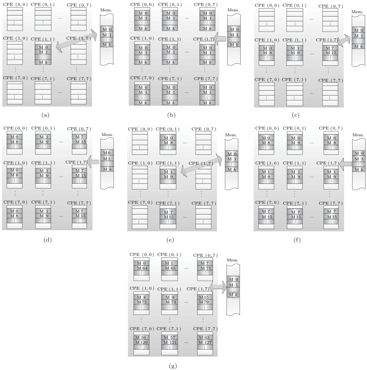
Fig.4. Patterns of data stream transfers. (a) Single CPE pattern. (b) Broadcast pattern. (c) Row pattern. (d) Broadcast row pattern. (e) Column pattern. (f) Broadcast column pattern. (g) Array pattern.
