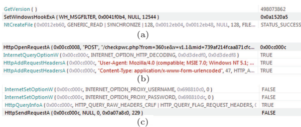
Fig.18. Call sequence fragment of M4. (a) M4 sets hook function with “SetWindowsHook” in Fig.5. (b) M4 builds socket handle with “Socket” and “Bind”, and then connects to remote server with “Connect” in Fig.7. (c) M4 sends the leaked data to remote server with “Send” in Fig.7.
