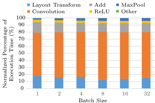
Fig.16. Time breakdown of ResNet-50 under different batch sizes under TensorFlow.
