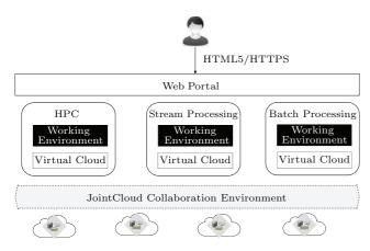
Fig.2. Virtual cloud for special purposes. HPC: hight performance computing
