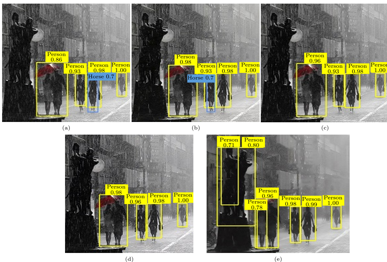
Fig.17. An application example of the proposed method for object detection in real rain weather. (a) Detection results of rainy images. (b) Detection results of deraining images of GCANet [21] . (c) Detection results of deraining images of NLEDN [16] . (d) Detection results of deraining images of PReNet [23] . (e) Detection results of deraining images of our method. More examples are displayed online ② .
