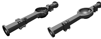
Fig.10. "Shaft": original CAD model and supershape representation.
