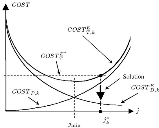
Fig.3. Cost curves for a given core  $C_k$ .
