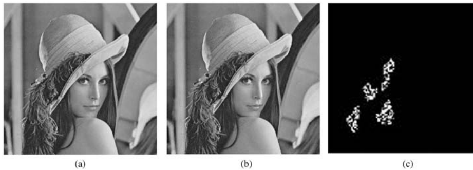
Fig.8. (a) Original image of Lena with bmp format. (b) Watermarked image. (c) Difference image which shows those areas which are tampered maliciously on hairs.
