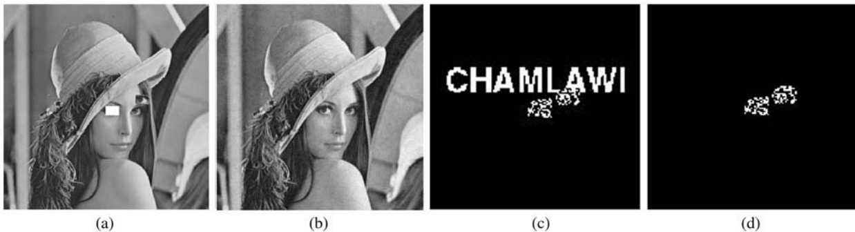
Fig.4. (a) Tampered image. (b) Recovered image. (c) Extracted watermark. (d) Difference between the original and extracted watermark.
