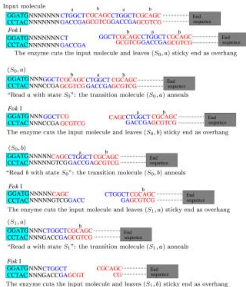
Fig.10. Several computational steps of the finite state machine.
