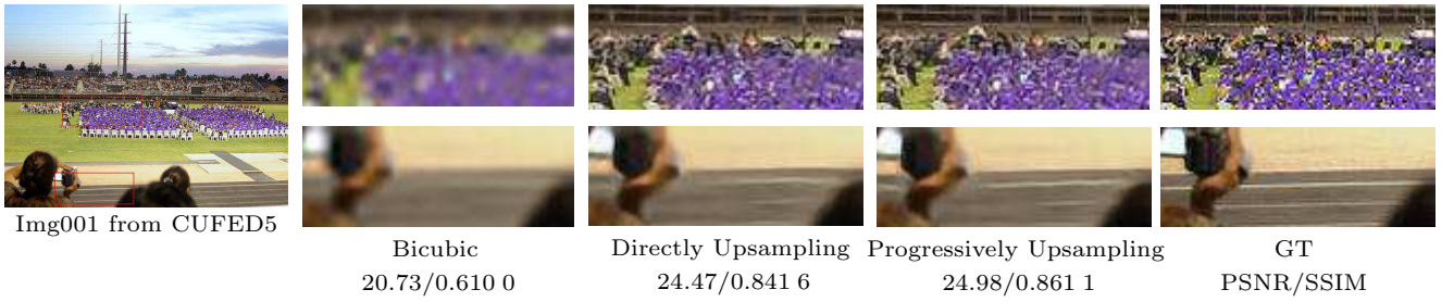
Fig.5. Visual comparison for ablation study of the progressively upsampling strategy. We show the close-up of the rectangle regions for better observation.
