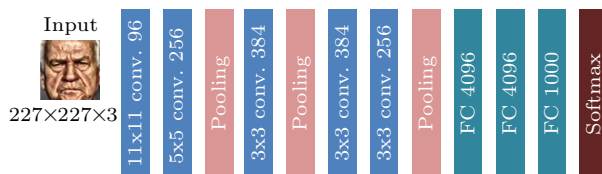
Fig.3. Architecture of AlexNet. It consists of five convolutional layers, some of which are followed by maximum pooling layers and then three fully-connected layers and finally a 1000-way softmax classifier.
