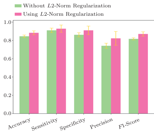
Fig. 7. Result of ablation study on L_2 -norm regularization method (mean±standard deviation) where the mean of five folds is drawn by the column and the standard deviation is presented by the yellow vertical line.
