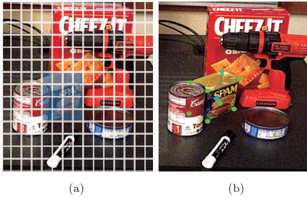
Fig.5. Simple example of our seg-reg two-stream network. (a) The segmentation stream labels every grid of the cropped image. (b) Offset vector and texture deviation of the center and corner points in the regression stream.
