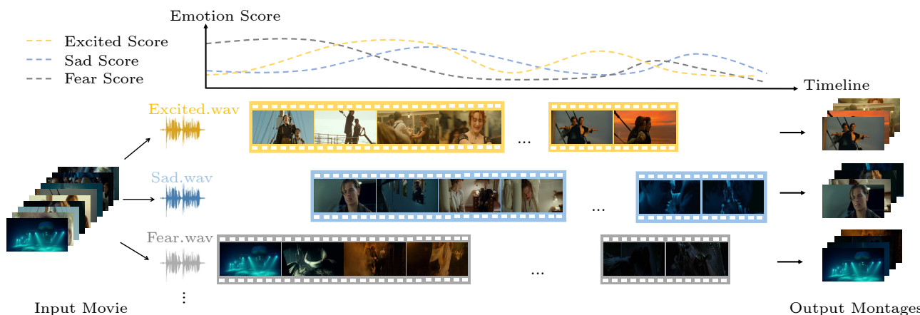
Fig.1. Emotion score based music-driven movie montage. When editing the same input movie with different background music, the corresponding emotion scores are completely different, and thus the final movie montages guided by different music are also distinct.
